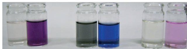
Figure 4. Colorimetric responses of receptor molecules 1b and 2b to addition of CN - (left hand pair), fluoride (middle pair) and chloride (null response control, right hand pair) in acetonitrile/methanol (>100:1) in the presence of tetrazolium violet.
